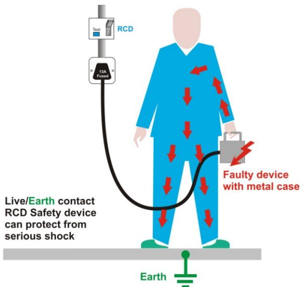
Figure 1: Protection against fatal electric shock by safety device.
