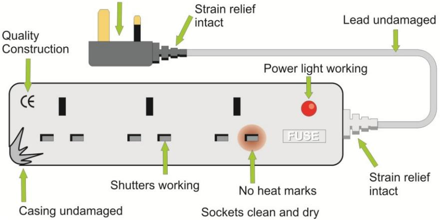
Figure 3: Extension lead with multiple socket outlet.
