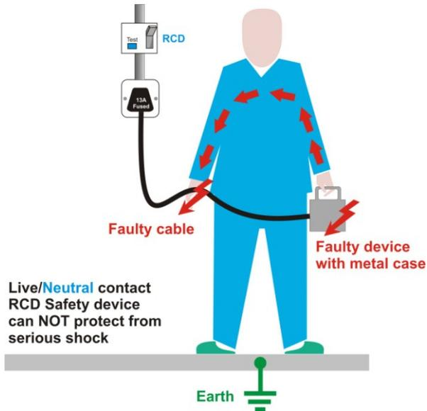
Figure 2: No protection against fatal electric shock.
